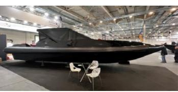
LoA: 14,40m | BoA: 3,70m | Weight (with engines): 6.500kg | Fuel Capacity: 1.500lt | Water Capacity: 200lt | Hull type: Tunnel Cat
